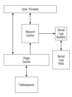
From the architecture diagram you can see the flow of data through the storage engine. All user thread activity begins with the record and page caches. The record cache is a memory cache used to maintain copies of both active and uncommitted records. The page cache is a memory cache used to hold database pages that are either being written to the database or being read from currently.
