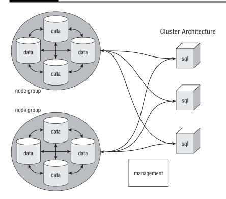
The management node is only needed during cluster startup. It can be made redundant by having more than one machine running the ndb\_mgmd process.
