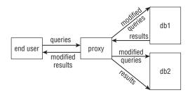
The end user connects to mysql-proxy, which may modify a query and send it to any of the backend addresses specified (in this example, dbl or db2). The database server then sends the results, which may be modified by the proxy before being sent back to the end user.
